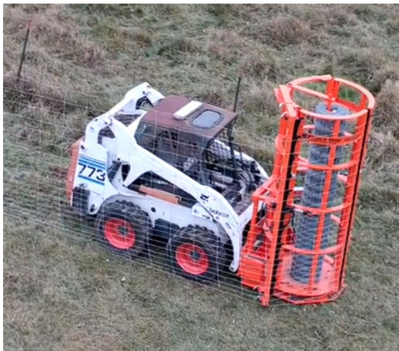
Figure 8. In 2025, MN WS installed a 6ft tall, woven wire, permanent fence with apron around a lambing pasture with historic depredation, using a new nonlethal initiative procured fence roller.
